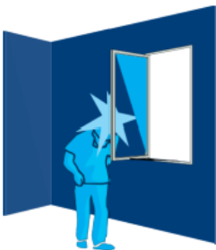
Risk of injury caused by sash impact when sashes are left open.
