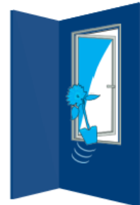
Danger of falling through if sashes are open.
