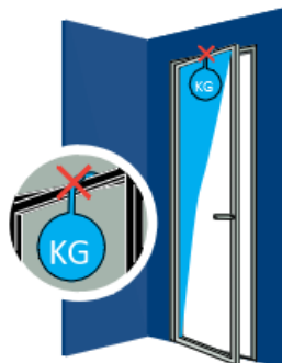
Load on the sashes or leaves can cause damage, deformation or destruction of individual elements..
