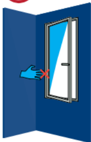
Risk of injury by getting stuck between window or door sash and frame.
